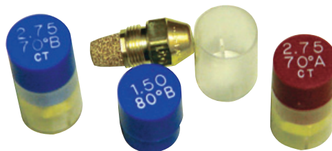
Nozzles need not be replaced every year if the fuel supply is kept clean and the oil filters are changed before each heating season.
