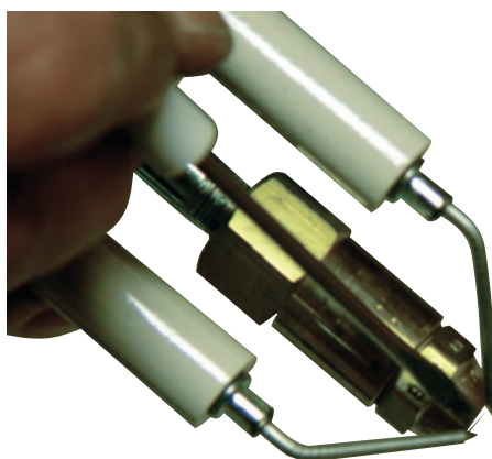
Electrode adjustment is often the cause of unit heater failure. Inspect electrodes for proper alignment and cleanliness.
