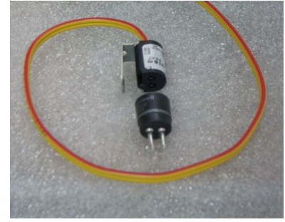
Cad Cell Eye Assembly. Sensor eye unplugged from mounting socket.
