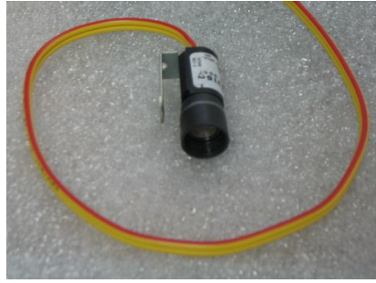
Cad Cell Eye Assembly removed from the igniter.
